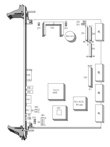
Figure 1.3: MIC-3358 jumper and connector locations.
